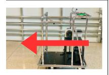
The cart must move this direction whether being pushed or pulled due to the swivel wheels.
