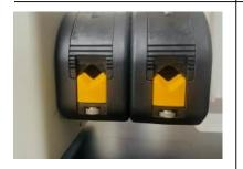
Component viscosities vary with different materials and these dials allow for adjustment if one component flows faster than the other.
