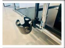
Attach drip cup holder to the cart. Allow mixing tube to hang directly above the drip cup. Use a disposable cup so you can throw it away at the end of the job.
