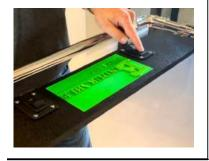
The button on the left of the control panel is the main power switch. It turns on the lights and readies the cart to turn on the motor.
