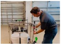
The wand attaches to the cart via the magnets. You may attach the wand to either of the front uprights and also to the rear left upright. Simply line up the magnets. This is considered single-user mode.
