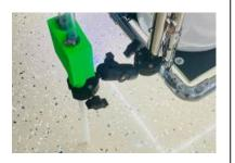
If using in single-user mode, keep the valve mixing tube off the floor to allow movement across the floor without the tube touching the floor.
