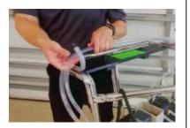
There are two hooks on the top platform which may be used to hold the excess tubing.
