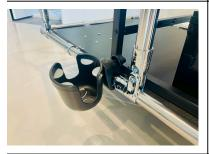
Attach the drip cup holder to the cart. Placement should allow the mixing tube to hang directly above the drip cup.
