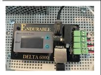
The circuit board is labeled for all cords and wires to attach properly. Please note there is a reset switch on the circuit board in case the circuit board is overloaded.
