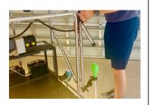
The wand may also be attached to the rear left upright, which allows the tube to drip into the drip cup when you are moving the cart.
