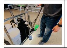
When you are ready to begin, turn on the pump and draw the material out of the buckets until the material is flowing through the valve with no air bubbles. It's good to pump into a waste bucket.
