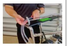
There are two hooks on the top platform which may be used to hold the excess tubing.
